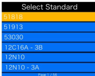
2. Use **MOVE** key to select Motorcycle battery model, The press **OK** key, the testing result will show one of these, as below: (Battery test result includes 5 types as following: )
