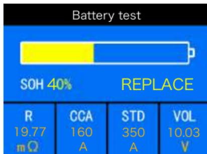
The battery is near to or already reached the end of the using life, replace battery otherwise, bigger danger will be followed.
