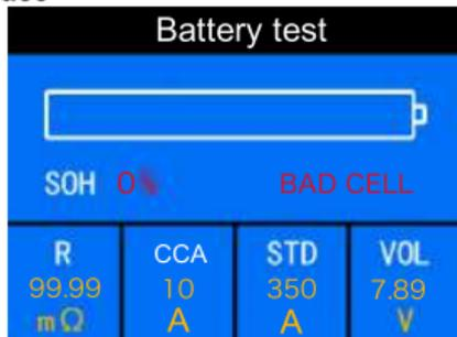
Battery interior damaged, bad cell or short circuit, replace battery.
